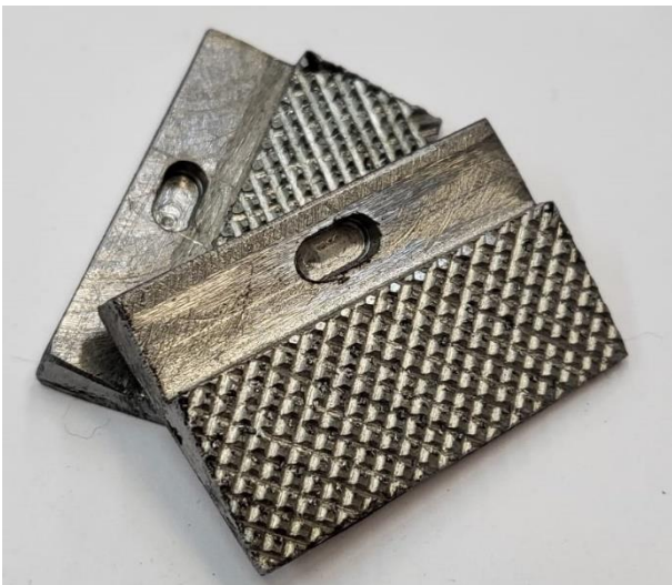
Figure 5: Serrated wedge grip inserts
