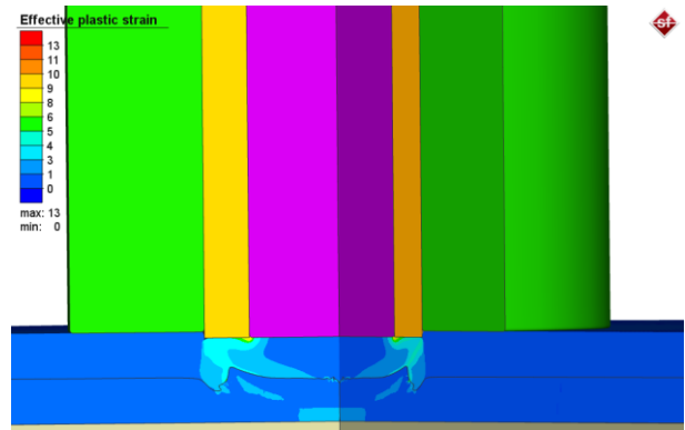
Figure 10: Residual strain distribution in plates
