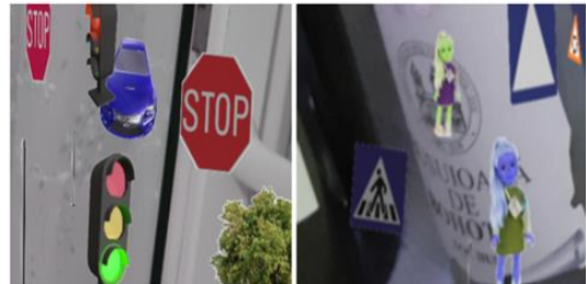
Figure 9: Output: 10,000 images with the given objects and text files describing the center and size of the bounding box for each object.
