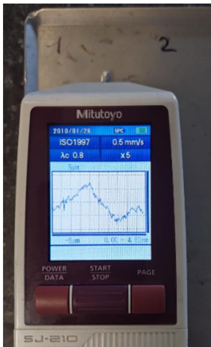
Figure 2.21. Measurement with the portable roughness
