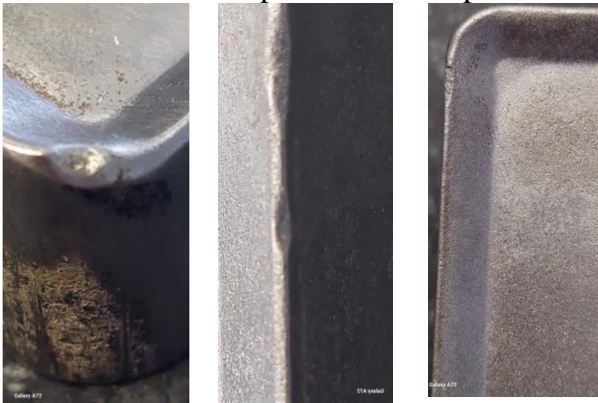
Figure 2.20. Contour defects of the punch
