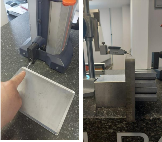
Figure 2.18. punch contour measurement
