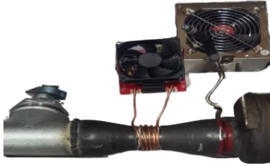
Figure 5: Assembly of the induction heating system in the injection area.
