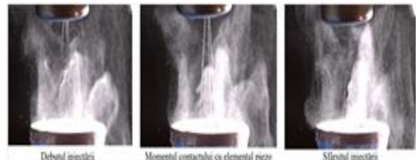
Figure 6: The distribution of AdBlue droplets in the case of an injection system on a piezoelectric element.
