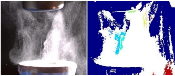
Figure 7: The distribution of AdBlue droplets in the piezoelectric system
