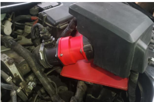
Figure 12: The intake pipe in the composition of the test system (equipment with manufactured item).
