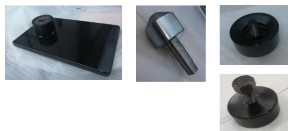
a) Base plate with support bushing and bearing b) Cone tree c) Fixing cover bottom view and top view
