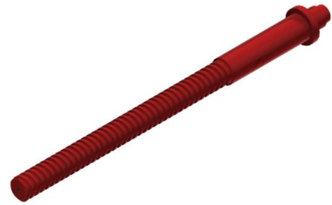
Figure 5: The final model of the trapezoidal screw, analogous to the square one.
