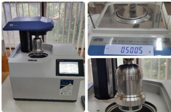
Figure 3. Sequences related to the determination of calorific value with the IKA C6000 calorimeter
