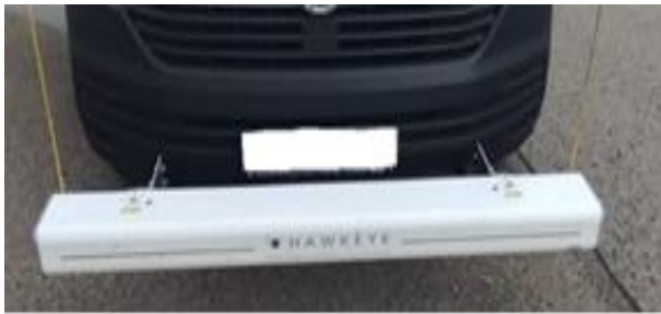
Figure 1: Hawkeye measuring equipment mounted on a transporter car type
