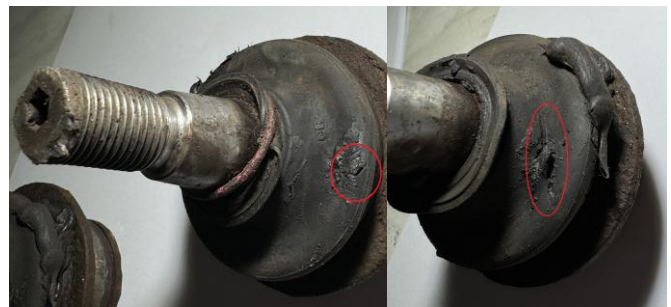
Figure 4: Worn ball joints of vehicle "E"
