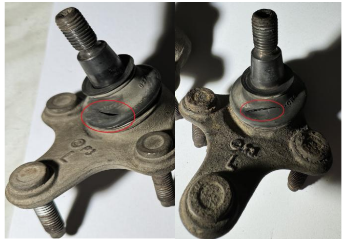
Figure 3: Worn ball joints of vehicle "B"
