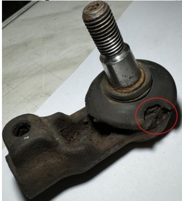
Figure 1: Ball joint of vehicle "F" with broken dust cover
