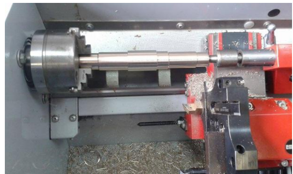
Figure 3: Straight shaft part on EMCO Concept Turn 55 CNC equipment [Susac,2017].
