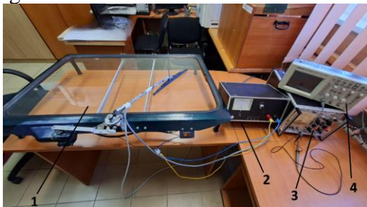
Figure 1: Experimental stand: 1. Wiper assembly – windshield; 2. Adjustable 12 V power supply; 3. Amplifier for strain gauge marks; 4. Digital oscilloscope.
