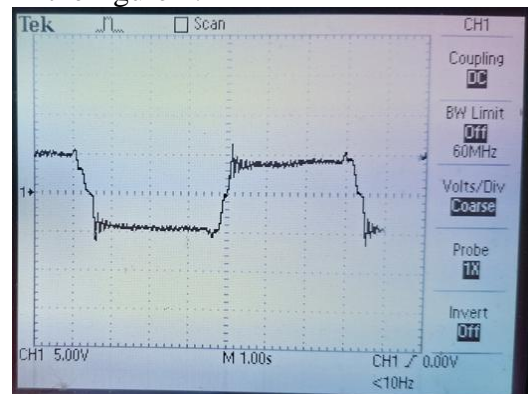
Figure 2: Example of a diagram recorded on an oscilloscope – Dry surface, voltage 4 V, period T = 1 s
