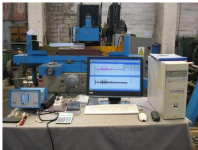
Figure 3: Have the equipment for acquiring results from the RPO200-AKS plan grinding machine from SC Vrancart Adj [Valea, 2019].
