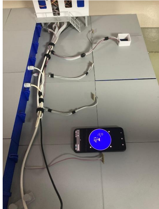
Figure 1: Measurement of the heel angle on the 1:25 scale model using a smartphone inclinometer application during the inclining test
